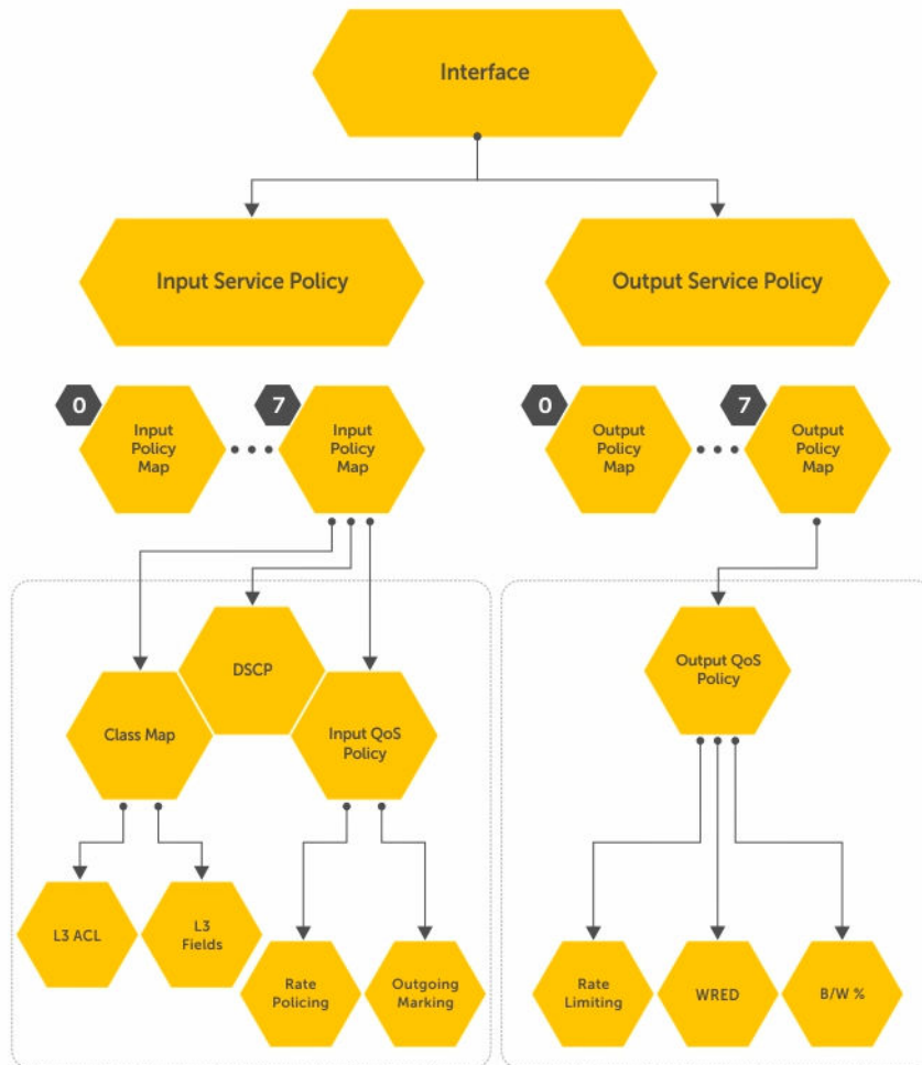
Figure 105. Constructing Policy-Based QoS Configurations
